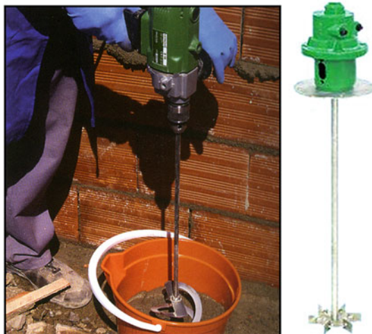
Fig. 3.45 Mixing with an electric mixer [35, 38]
