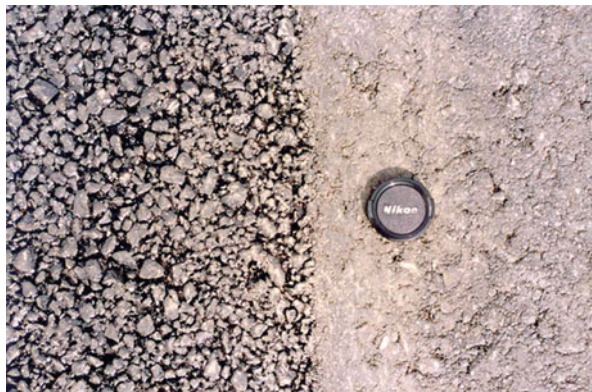
Fig. 5.7 Texture of the pavement surface in porous asphalt ( left ) and asphalt concrete ( right )
