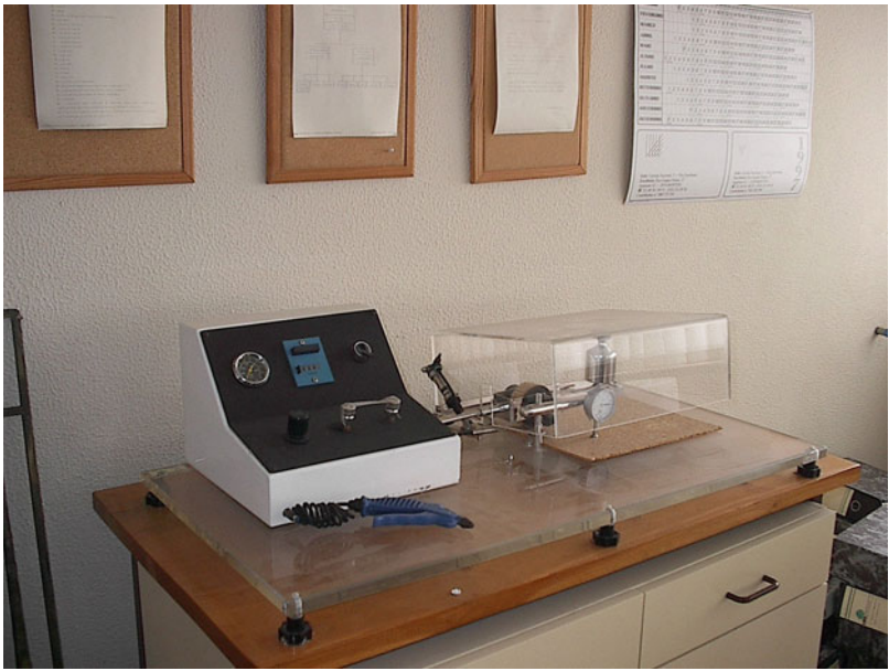
Fig. 13.15 Abrasion test for cork flooring
