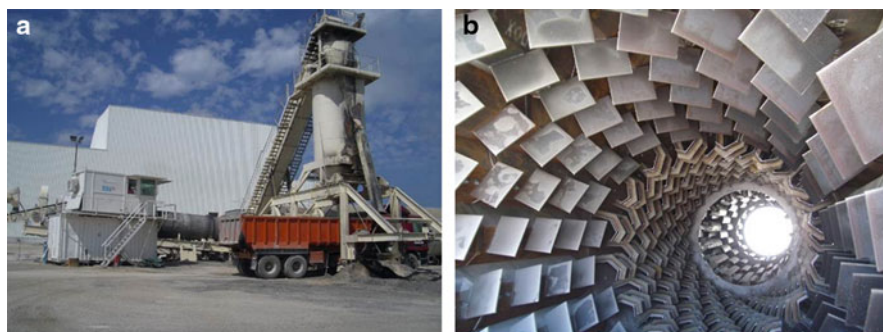
Fig. 5.8 Drum mix plant: (a) general view; (b) inside part of the drum mixer
