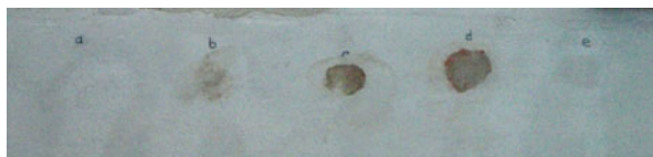
Fig. 3.10 Dirt resistance tests using staining products [13]
