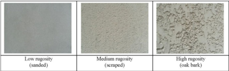
Fig. 2.29 Rugosity of premixed mortar coatings [42]
