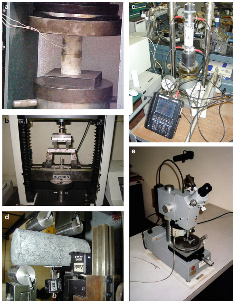
Fig. 9.11 Common mechanical test: (a) uniaxial compression strength test in cylindrical specimens; (b) flexural strength under constant moment; (c) dynamic elastic modulus; (d) fracture toughness; (e) microhardness test
