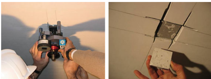
Fig. 3.7 Pull-out test and adhesive failure in the interface between the ceiling's gypsum coating and the concrete substrate
