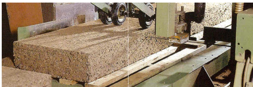
Fig. 13.7 Cutting the block into boards
