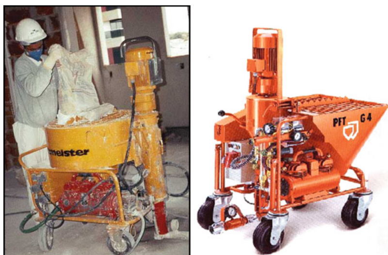
Fig. 3.46 Mixing with the spraying device itself [39, 40]
