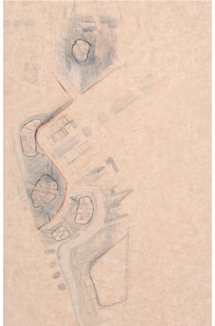
Sketch layout by Beigel showing the Stone units inserted into the existing wetland area as conceived for the purpose of creating a distinctive group of office buildings. These were to be closely related to the existing watercourses of the immediate wetland area, linked by connecting bridges.
