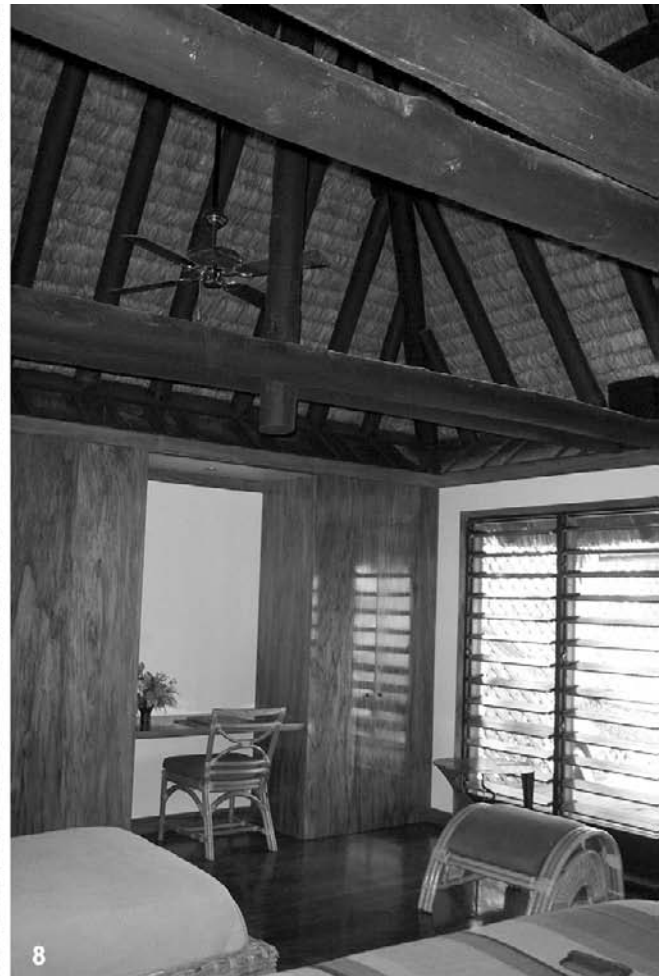
Figures 4.1.7–8 The design of individual guest units is based on traditional Fijian houses. Their high cathedral ceilings, lightweight thatched roofs and generous louvered windows on both long sides ensure an excellent thermal environment even without air-conditioning.
