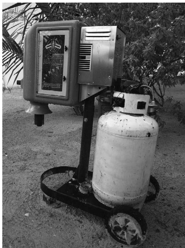
Figure 4.6.7 A 'mosquito magnet', which attracts and captures mosquitoes, helps to control the insect problem on site.
