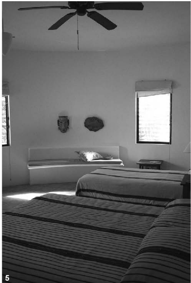
Figures 4.6.4–5 Second-storey units benefit from high cathedral ceilings allowing hot air to rise under the roof; ground floor units have their thermal environment shaped by the openness of the plan and staying permanently in the ‘shade’ of the upper floor.
