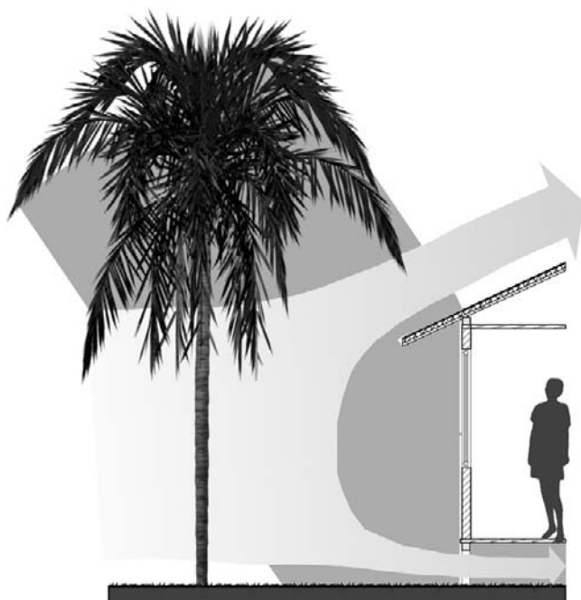
Figure 3.7 High-branched trees, such as palms, provide shade and let the air flow freely around the building.
