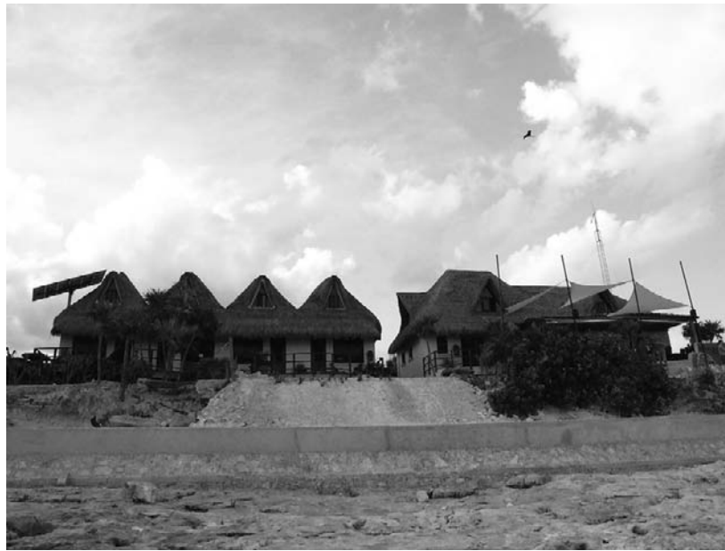
Figure 4.5.12 The two parts of the resort – the guest unit one (on the left) and restaurant/office (on the right) – are separated, which, together with background noise from the breaking waves, ensures favourable acoustic conditions.
