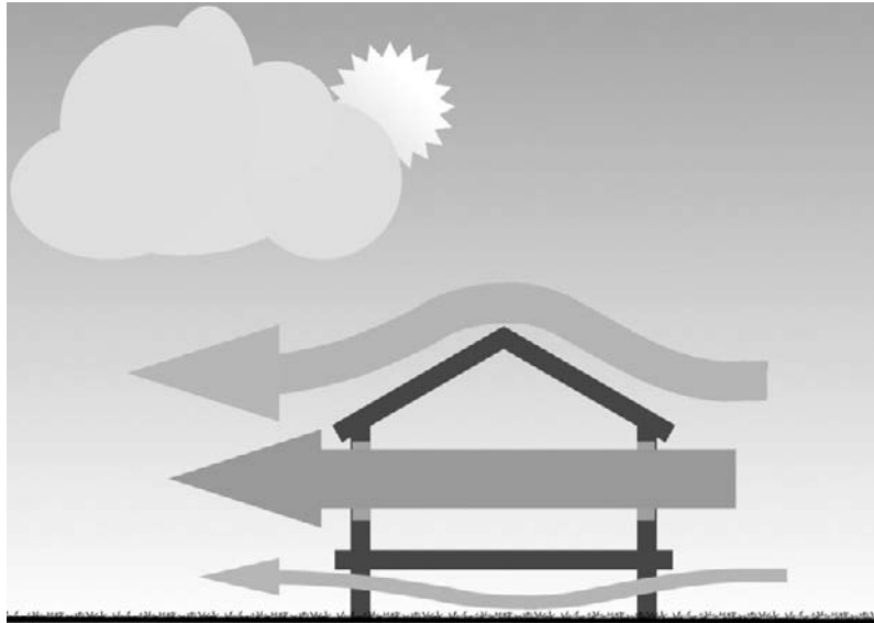
Figure 3.25 Cooling the building with flowing air.
