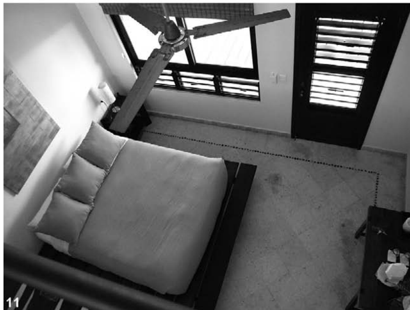
Figures 4.5.10–11 Room height allows for vertical air movement and sensible cooling through stack effect ventilation making the indoor environment thermally comfortable.
